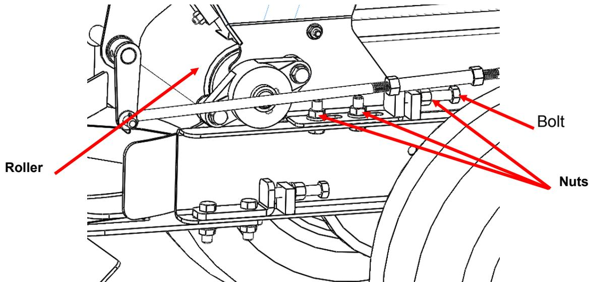
**The spreader does not move forward or does so, with difficulty.**
