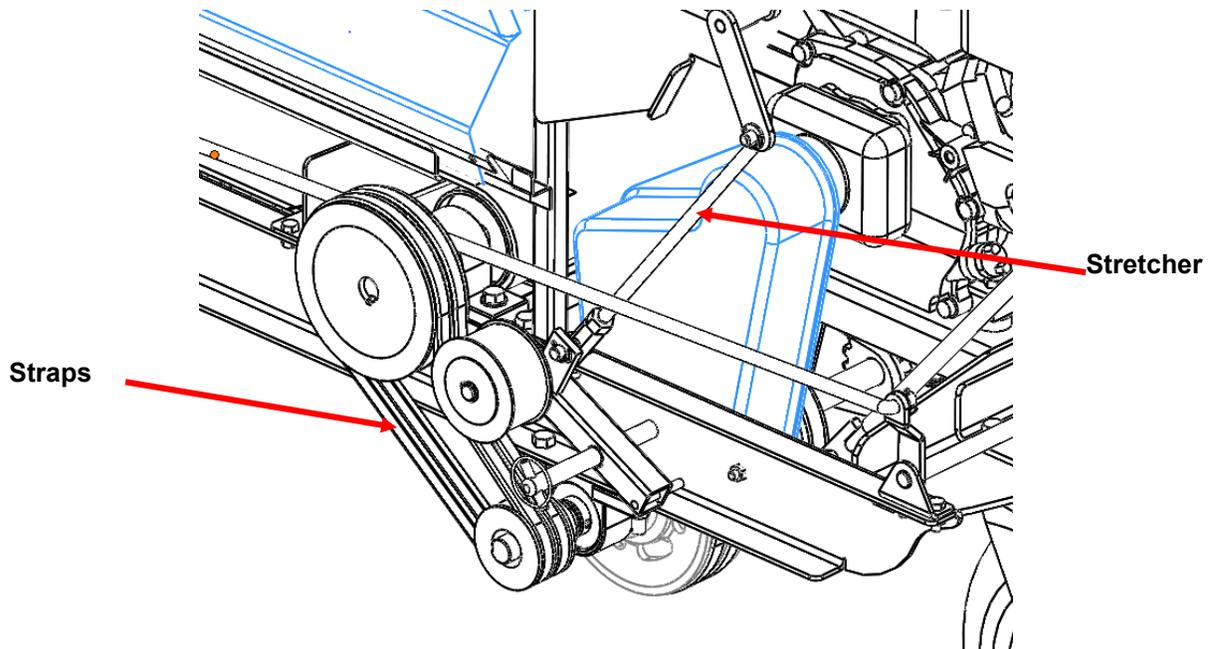
If the tension is incorrect, adjust the stretcher of the conveyor, 1/8 inch at a time.
